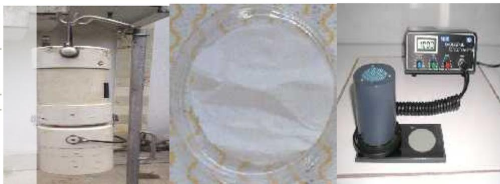
Gambar 2(a) Mini Volume (MiniVol) Portable Air Sampler
