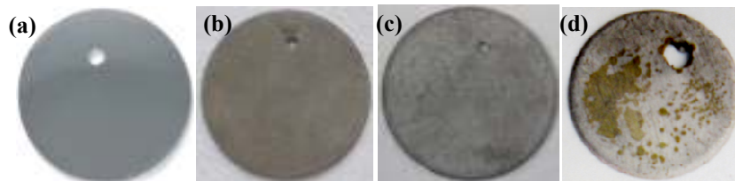
Figure 3. Photograph of the (a) original specimen (b) untreated specimen (c) treated specimen in silicate-based corrosion inhibitor (d) treated specimen in lignocelluloses corrosion inhibitor.
