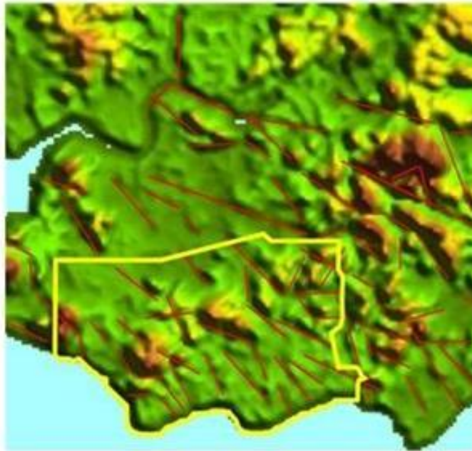
Figure 5. Map of interpreted lineament using DEM data.
