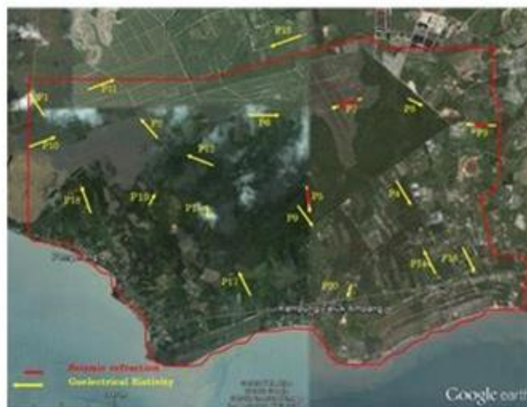
Figure 6: Survey lines within the area captured by Google.
