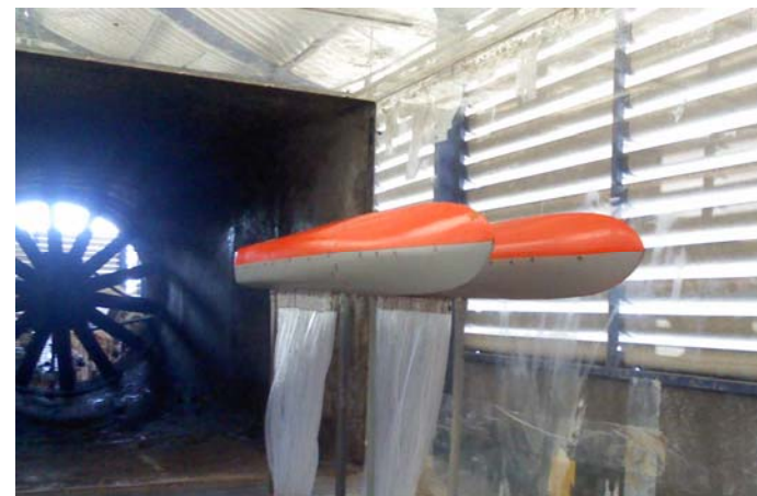
Figure 2. Test set-up model of catamaran with no turbulence stimulator in the wind tunnel.
