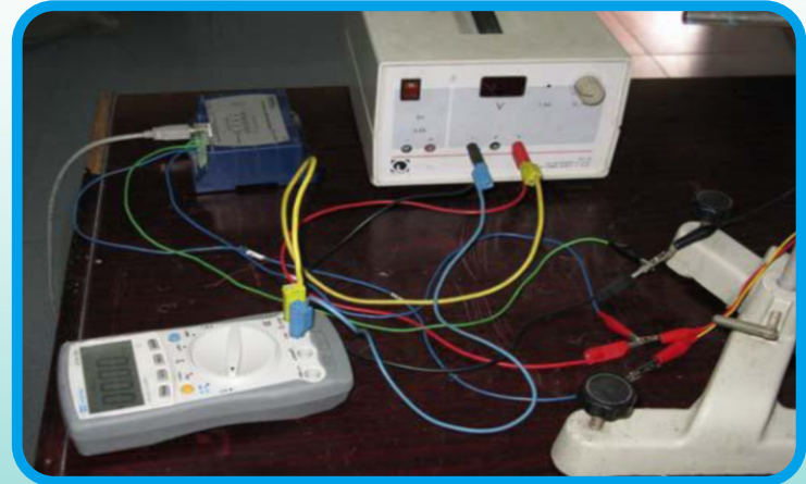
Gambar . Pengukuran statis sensor suhu PTC
