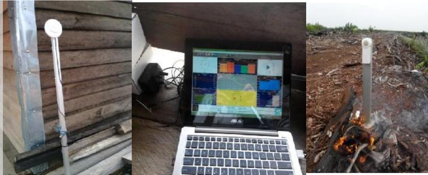
**Gambar 4.93** Pemasangan transmitter, aplikasi accurate peat fire detection (APF detection) dan sensor api di lokasi penelitian
