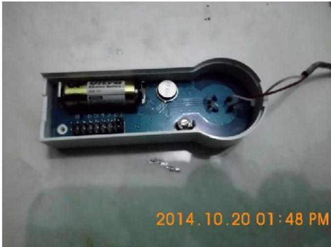
Gambar 4.14 Modul Rangkaian Transmitter Diberi Battery Alkaline 12v
