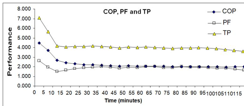
Figure 4 Performance (COP, PF, TP) of hybrid refrigeration machine
