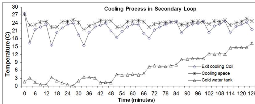
Figure 7 Temperature variation of exit cooling coil, cooling room and cold water tank (cold water tank as TES ice on coil)
