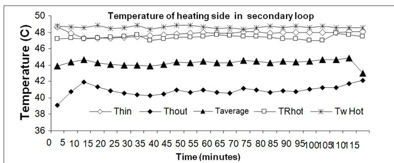
Figure 5 Temperature variation of heating side in secondary loop
