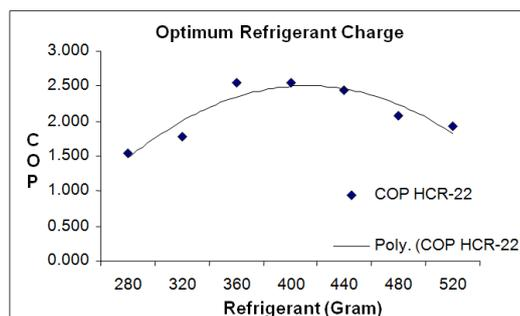
Figure 2 Coefficient of Performance (COP) vs refrigerant charge (gram)
