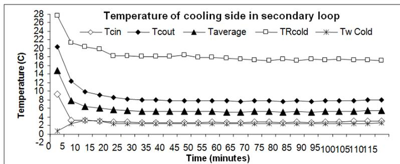
Figure 6 Temperature variation of cooling side in secondary loop
