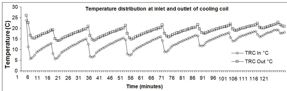
Figure 8 Temperature variation of inlet and outlet of cooling coil (cold water tank as TES ice on coil)
