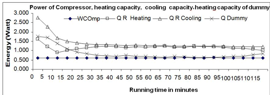
Figure 3 Energy of compressor, heating and cooling vs running time (minutes)
