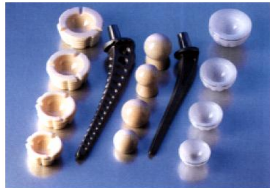
Figure 3. Medical-grade \text{Al}_2\text{O}_3 used in total hip replacement [1].
