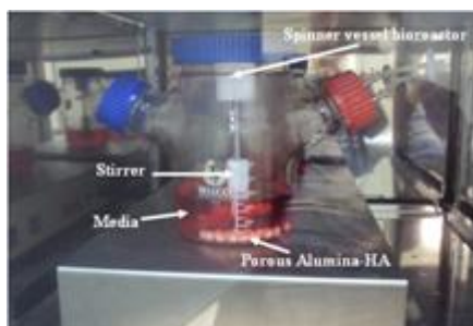
Figure 1. Vero cell culture in the spinner vessel bioreactor with controlled parameters
