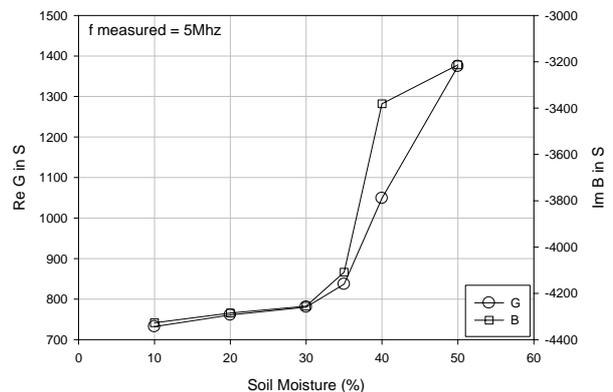
**Figure 6. The Real  $G$  and imaginary part  $B$  of soil impedance shown dependency of soil moisture**
