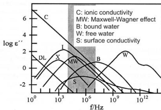
**Figure 1. Dielectric dispersion in wet soil [Hasted, 1973]**
