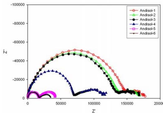
**Figure 4. Semi circle impedance of soil moisture measurement**
