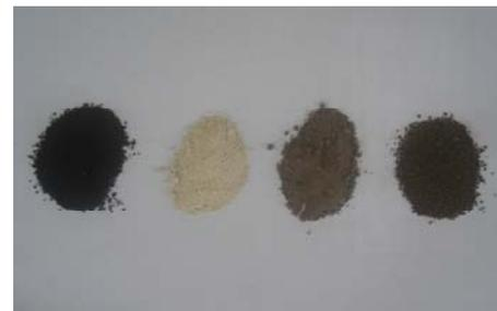
**Figure 2. Different soil samples, after preparation using oven dried**
