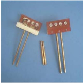
**Figure 3. Soil sensor electrode**
