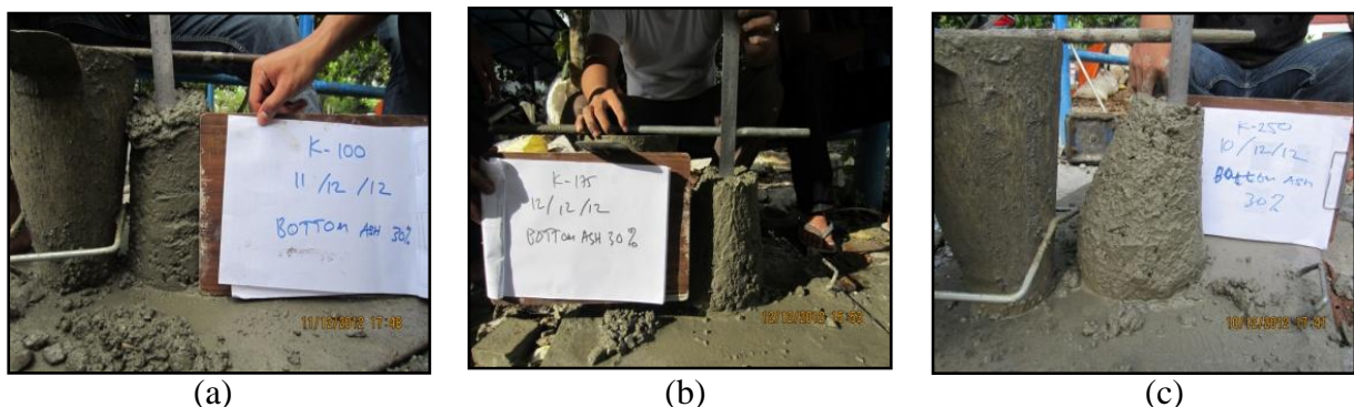
Gambar 1. (a) Pengujian slump K-100 BA 30% (b) Pengujian slump K-175 BA 30% (c) Pengujian slump K-250 BA 30%
