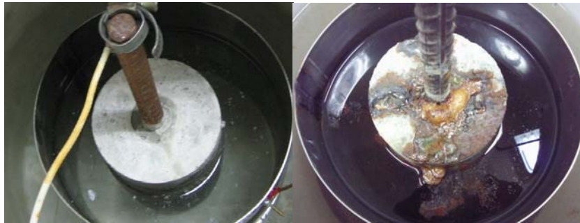
Figure 8. Appearance of OPC concrete specimen (left: before test started, right: after crack).
