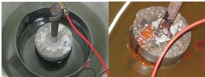
Figure 9. Appearance of geopolymer concrete specimen (left: before test started, right: after first rust observed).
