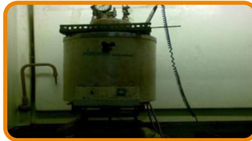
Pengoperasian Alat Saat Sintesis ZSM-5
