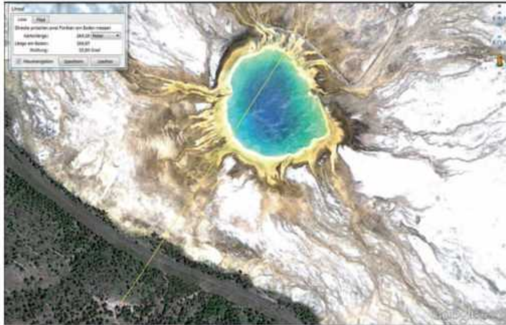
Figure 1. Snapshot from (German) Google Earth (© 2011 Google) of Grand Prismatic Spring in Yellowstone National Park with surroundings. The window with the ruler gives two measures of the line, one on-map (top value 269.29 m) and one on-ground (bottom value 269.87 m). For the lower point, Google Earth gives elevation: 2234 m, latitude: 44^{\circ} 31' 24.68'' and longitude: 110^{\circ} 50' 23.49'' . For the upper one we have elevation: 2218 m, latitude: 44^{\circ} 31' 32.00'' and longitude: 110^{\circ} 50' 16.84'' .
