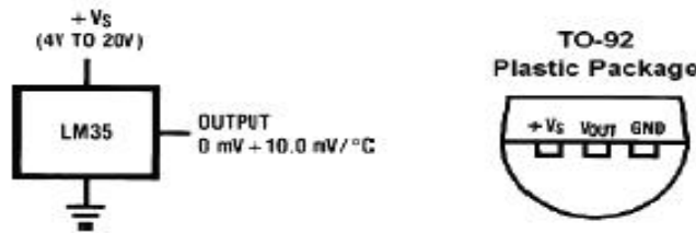
Gambar 2.8 Simbol dan tata letak terminal Sensor LM35 (National Semiconductor Corporation, 1999)
