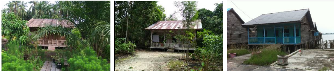
Figure 6. Akit Meranti house with leaves roof (a) wall board with zing (b) glass windows (c)
