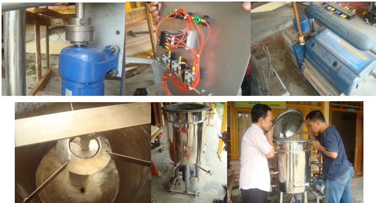
Gambar 8. Proses Assembly dan Running Test Vacuum Evaporator di UKM Al-Hikmah
