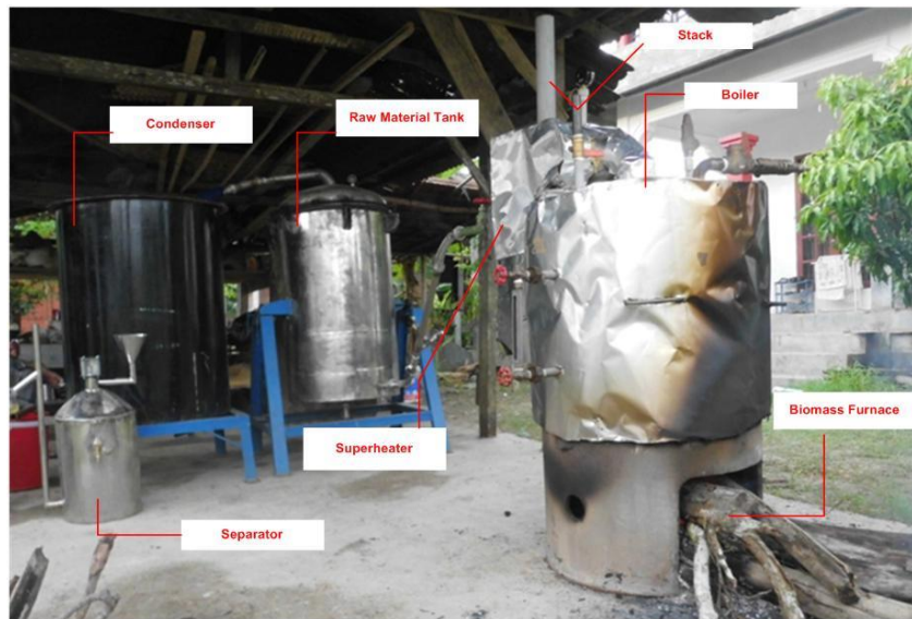
Figure 2. Performance test of patchouli oil steam distillation equipment
