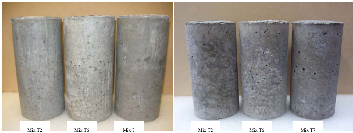
Figure 6. Visual appearance of mix T2, T6, T7 before and after exposure to the wetting drying cycles test (left: before exposure, right: after exposure).
